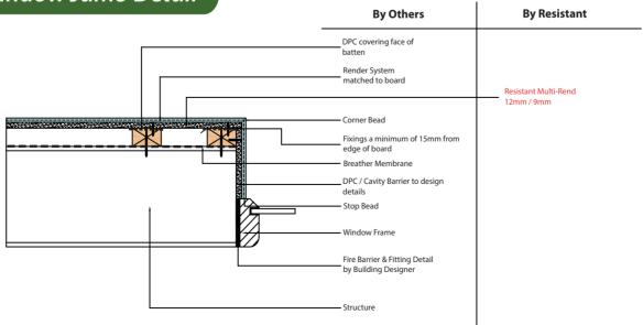
\*Multi-Rend board must be dry, clean & free from dust etc before a render is applied to the board\*
