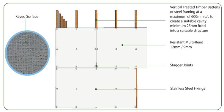
\*Multi-Rend boards must be fitted horizontally to create a brick bond effect. This will stagger joints and increase the strength of the overall boards. If fixed at 300mm centres 27 fixings per board will be required.\*
