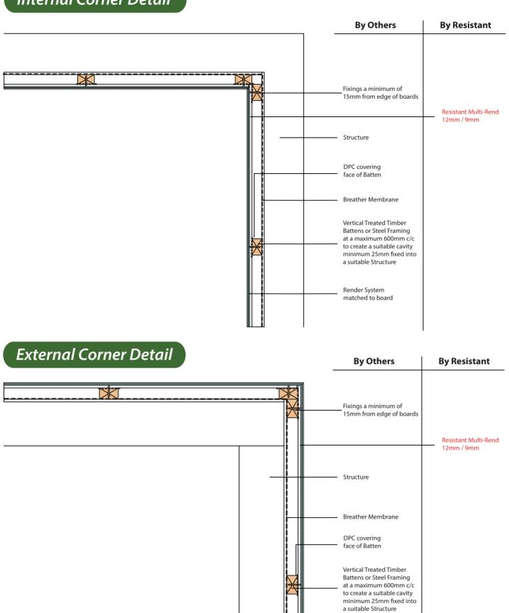
\*Multi-Rend board must be dry, clean & free from dust etc before a render is applied to the board\*
