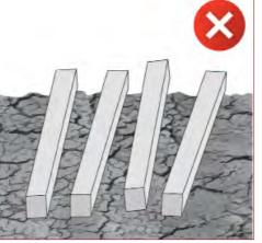
A structurally sound sub frame must be installed ensuring there is no movement prior to fixing boards to the joists. A 5% fall to allow water to drain and a min 100mm free air space between the boards and the ground beneath to allow sufficient airflow to prevent the build up of moisture is essential.
